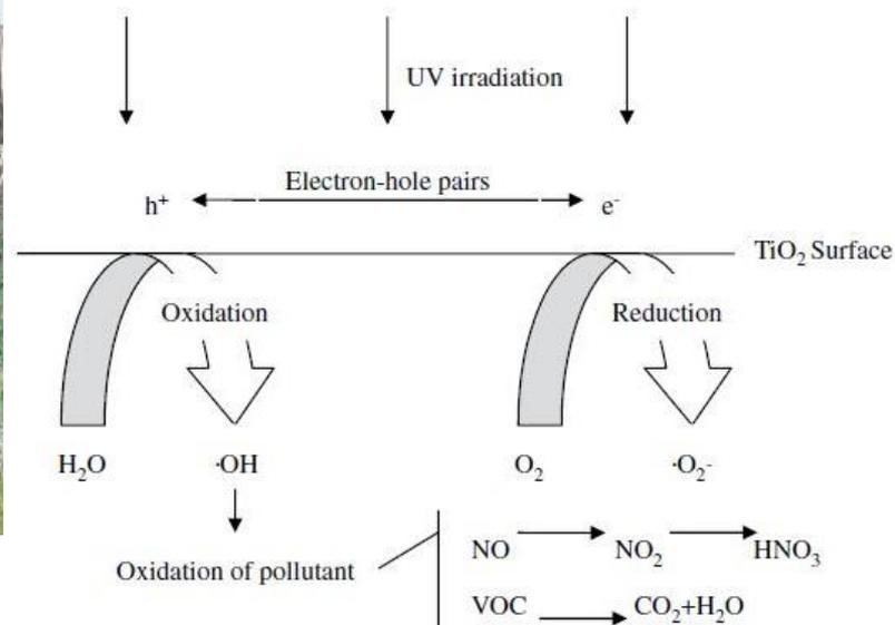
Pollution removal mechanism of  $\text{TiO}_2$  photocatalysis
